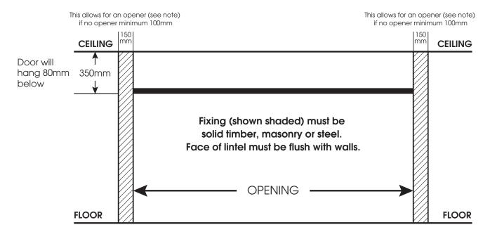
NOTE: High wind doors will require another 50mm of side fixing if an opener is being fitted.
