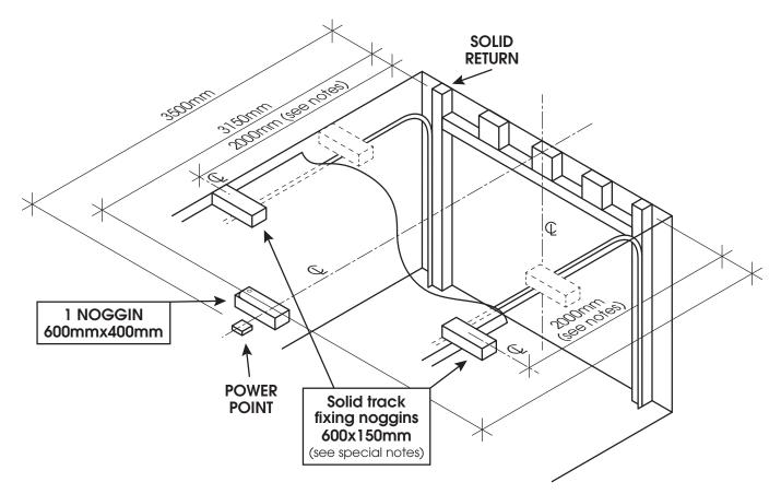
**NOTES:** Doors higher or wider than 2285mm high x 5200mm wide and all wind rated, insulated or special P7D doors will require two intermediate fixings at 1000mm (see page 2 for other sizes).
