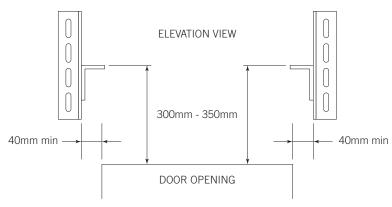
To determine the centre line of the shaft to the inside of the bulkhead, refer to the door bundle schedules on page 8:
