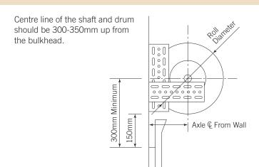
To locate bracket position: Measure the bottom rail. Add 50-100mm to the bottom rail measurement.
