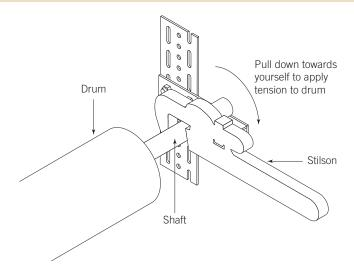
To put tension on door place stilsons on shaft from inside. Now pull down back towards you from inside of the drum. As the door tension increases the shaft will want to slip backwards. Hold shaft in place with stilsons and gently tighten U-bolt nuts further. Proceed with applying tension until the curtain rises approximately 100 - 200mm from the floor. At this distance the tension should be correct. Then tighten U-bolts on both ends.
