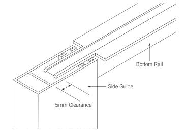
Fit side guide to the wall (bottom rail to have 5mm clearance between guide and slat each side of opening).
